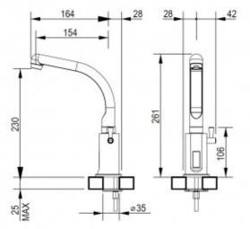
Electronic mixer with a mixer for two 1/2 &HASH39; connections for cold and hot water, adapted for installation on a wash basin. The outer part of the faucet is made of chrome-plated brass. The battery is available in two power variants:
