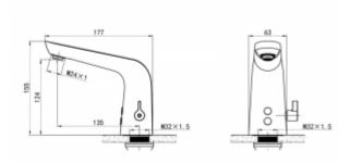
Touchless basin faucet with mechanical mixer, designed for public spaces. Automatically activated by a proximity sensor (infrared), it ensures hands-free operation, a high level of hygiene, and water savings.
