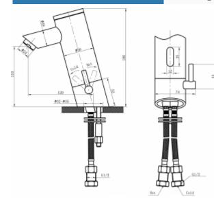
Contactless stainlees steel battery. Possibility to conect hot, cold and pre-mixed water. Possibility of smooth water temperature Designed for public facilities and homes.
