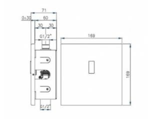
A flush-mounted electronic battery for urinal sets. The tap has one 1/2 connection for cold or mixed water. The outer casing of the product is made of chrome-plated AISI 304 stainless steel. It is worth adding here that the correct operation of the battery is possible only when connected to water free of impurities. An indispensable element for the correct operation of the product is a filter (must be installed by yourself).
