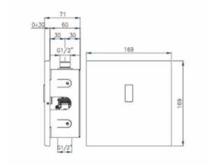
A flush-mounted electronic battery for urinal sets. The tap has one 1/2 connection for cold or mixed water. The outer casing of the product is made of chrome-plated AISI 304 stainless steel. It is worth adding here that the correct operation of the battery is possible only when connected to water free of impurities. An indispensable element for the correct operation of the product is a filter (must be installed by yourself).
