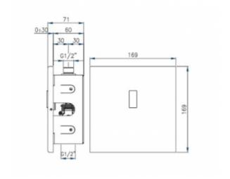
A flush-mounted electronic battery for urinal sets. The tap has one 1/2 connection for cold or mixed water. The outer casing of the product is made of AISI 304 stainless steel. It is worth adding here that the correct operation of the battery is possible only when connected to water free of impurities. An indispensable element for the correct operation of the product is a filter (must be installed by yourself).
