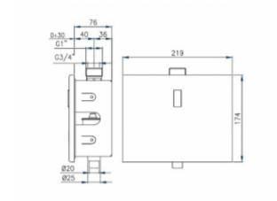
Flush-mounted electronic flush faucet. The tap has an adjustable connection, which means that there are two options of connection 1 "and 3/4 &HASH39;- for manual setting.
