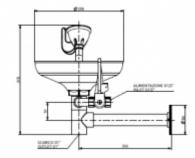
Double eyelet with a bowl made of high quality ABS plastic. Wall mounted. Operated with a side lever.
