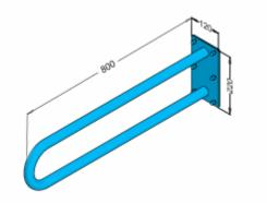
Handrail for disabled people, arched, fixed, 800 mm long, generalpurpose, made of 32 mm diameter carbon steel tube, white powder coated. We use this type of handrail in the washbasin, shower, and toilet area.
