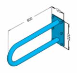
Handrail for disabled people, arched, fixed, 500 mm long, generalpurpose, made of 32 mm diameter carbon steel tube, white powder coated. We use this type of handrail in the washbasin, shower, and toilet area.
