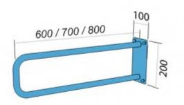
Handrail for disabled people, arched, fixed, 600 mm long, generalpurpose, made of 25 mm diameter carbon steel tube, black powder coated. We use this type of handrail in the washbasin, shower, and toilet area.
