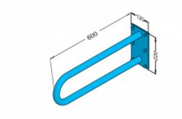
Handrail for disabled people, arched, fixed, 600 mm long, generalpurpose, made of 32 mm diameter carbon steel tube, white powder coated. We use this type of handrail in the washbasin, shower, and toilet area.
