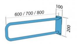
Handrail for disabled people, arched, fixed, 700 mm long, generalpurpose, made of 25 mm diameter carbon steel tube, black powder coated. We use this type of handrail in the washbasin, shower, and toilet area.
