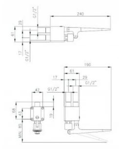
Foot tap, time-controlled tap with single 1/2 &HASH39;connection for cold or mixed water. The pedal actuation reduces the need for the user&HASH39;s hand. Foot-operated taps are most often used in gastronomy or surgery where special attention is paid to the sterility of the hand. The 9060 battery is a product that is ideally suited for use by disabled people or children. Wall or floor mounting possible.
