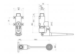
Foot or time mixer for cold or mixed water. A special battery operated by a pedal prevents the user&HASH39;s hands from coming into contact with the device. Used in gastronomy or surgery where special attention is paid to hand sterility. Wall or floor mounting possible. It can be used as a time battery for people with disabilities.
