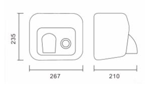
Professional hand and hair dryer, activated at the touch of a button. Intended for swimming pools, hospitals, medical, treatment and dental offices. The casing of the offered dryer is made of stainless steel, which is highly resistant to vandalism. In addition, the steel housing is waterproof and has an IPX1 protection.
