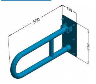
Arch hand-tilt, wall, for disabled people, 500 mm long, generalpurpose, made of polished stainless steel tube or matt 32 mm diameter. We use this type of handrail in the washbasin, shower, and toilet area.
