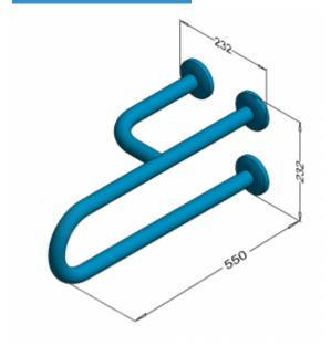
Left basin handrail for disabled people, 550 mm long, generalpurpose, made of polished or matt stainless steel tube, 32 mm diameter. We use this type of handrail in the washbasin. The handles are equipped with masking rosettes with a click system, which allows mounting the masking rosette without the use of mounting glue.
