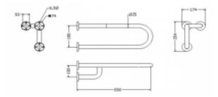
Right basin handrail for disabled people, 550 mm long, generalpurpose, made of stainless steel tube, 25 mm diameter. We use this type of handrail in the washbasin. The handles are equipped with masking rosettes with a click system, which allows mounting the masking rosette without the use of mounting glue.
