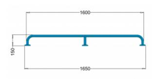
The 1600mm straight handrail is a product that is a basic mobility aid for disabled people. The offered handrail is made of a pipe with a diameter of 32 mm and a pipe wall thickness of 1.5 mm, made of AISI 304 stainless steel, in two variants as to the finish of the outer coating. The available outer shell finishes are:
