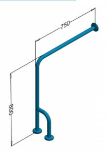
Wall and floor left mounted handrail for disabled people, length 750x800mm, general-purpose, made of polished stainless steel tube or matt 32 mm diameter. We use this type of handrail in the washbasin, shower, and toilet area. The handles are equipped with masking rosettes with a click system, which allows mounting the masking rosette without the use of mounting glue.
