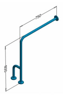
Right wall and floor mounted handrail for disabled people, length 750x800mm, general purpose, made of polished stainless steel tube or matt 32 mm diameter. We use this type of handrail in the washbasin, shower and toilet area. The handles are equipped with masking rosettes with a click system, which allows mounting the masking rosette without the use of mounting glue.
