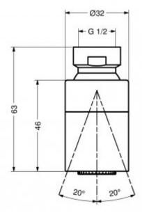
Made of chrome-plated brass. The head strainer is made of plastic with rubber nozzles, which make it difficult to settle the stone and facilitate its leveling.
