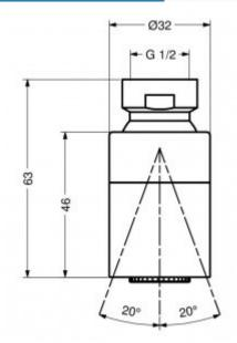
Made of chrome-plated brass. The head strainer is made of plastic with rubber nozzles, which make it difficult to settle the stone and facilitate its leveling.
