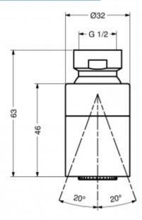
Made of chrome-plated brass. The head strainer is made of plastic with rubber nozzles, which make it difficult to settle the stone and facilitate its leveling.
