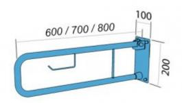
Handrail for people with disabilities arched, tilting, a wall with space for paper, 800 mm long, general-purpose, made of 25 mm diameter carbon steel tube, powder-coated, white. We use this type of handrail in the wc area.
