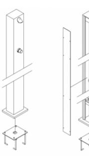
Column shower set made of AISI 316 stainless steel, adapted for outdoor-floor installation. The shower set 9231 is equipped with a ceramic mixer. Standard water flow bowls are approximately 30-50 seconds ± 1 second. The flow system is enriched with a safety device that automatically shuts off the water flow after 15 seconds at a pressure of 3 bar.
