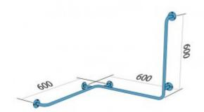
Left handrail for the bathtub left-hand shower mounted to the wall 600x600x600 mm long, made of carbon steel tube with a diameter of 25 mm powder coated white. We use this type of handrail in the bathtub and shower area.
