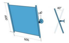
Tilting mirror for disabled people in a side frame, made of black enameled carbon steel. The mirror frame has a size of 600 x 600 mm and is made of a steel tube with a diameter of 25 mm and a wall thickness of 1.5 mm. The mirror sheet, on the other hand, has dimensions of 546 x 440 mm, and the thickness of its coating is 120 μ. The presented mirror is designed for wall mounting in the washbasin area.
