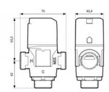
Thermal mixer with G1 connections and with hald screw for cold and hot water with an element regulating the temperature. The temperature is adjusted when the knob is used. The knob has a double scale, the outer one shows the half-scale, the inner one shows degrees Celsius.
