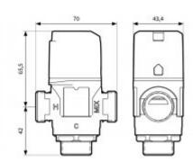
Thermal mixer with G3/4 connections, with half screw for cold and hot water with an element regulating the temperature. The temperature is adjusted when the knob is used. The knob has a double scale, the outer one shows the half-scale, the inner one shows degrees Celsius.
