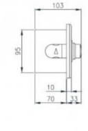
Mounting box made of stainless steel. Designed for mounting time battery 9005, 9005P.
