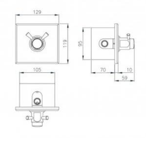
Mounting box made of stainless steel. Designed for mounting 9005MIX PLUS valve
