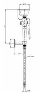
Single eyelet, straight, attached to the wall.
