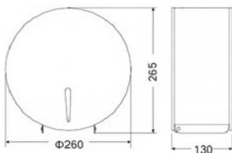
Toilet paper dispenser, made of stainless steel AISI 304 in two surface finishes:
