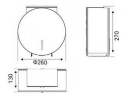
Toilet paper dispenser made of stainless steel. Matte finish. Capacity: 1 roll. Lockable with a key. Vandal. It has a window for viewing the remaining amount of paper.
