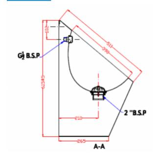
Stainless steel urinal, designed for surface-mounting. Product designed for public toilets exposed for damages, Suggested siphon SHC4.
