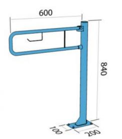
Arched handrail for people with disabilities, floor mounted. With space for paper. 600 mm long, general-purpose, made of 25 mm diameter carbon steel tube, powder-coated in white. We use this type of handrail in the wc area.
