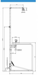
Rescue platform with integrated safety spray and eyelet. The water is activated immediately after entering the platform.
