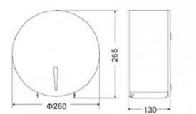
General-purpose toilet paper dispenser. The offered feeder is made of AISI 304 stainless steel in a black finish. The stainless steel 1.4301 used is a universal material that is often used in the production of sanitary products. It is highly resistant to vandalism, corrosion, rust, and most oxidizing acids.
