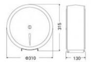
Toilet paper dispenser made of stainless steel. Matte finish. Capacity: 1 roll up to 300mm in diameter. Lockable with a key. Vandal. It has a window for viewing the remaining amount of paper.
