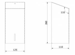
Toilet paper dispenser in sheets made of stainless steel. Matte finish. Capacity: 400 sheets. Lockable with a key. Vandal. It has a window for viewing the remaining amount of paper.
