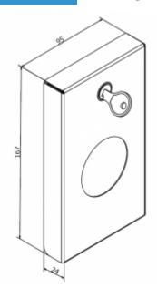
Sanitary bag dispenser made of AISI 304 stainless steel. The steel used in the production is highly resistant to corrosion, rust and moisture. This means that the offered feeder can be placed in a room exposed to increased humidity.
