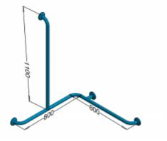
Right angular handrail for disabled people, 800 x 800 x 1100 mm long, general-purpose, made of polished or matt stainless steel tube, fi32mm. We use this type of handrail in the washbasin, shower, and toilet area. The distance of the handrail from the wall to the center of the tube is 90 mm.
