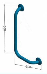
Right angular handrail for disabled people, 300 x 600mm long, generalpurpose, made of polished or matt stainless steel AISI 304 tube, fi 32mm. We use this type of handrail in the washbasin, shower, and toilet area. The handles are equipped with masking rosettes with a click system, which allows mounting the masking rosette without the use of mounting glue. The distance of the handrail from the wall to the center of the tube is 90 mm.
