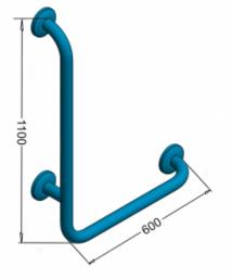
Right angle handrail, "L" type, for the disabled, for general use, made of a 32 mm diameter tube, made of AISI 304 stainless steel. The steel used in the production is highly resistant to corrosion, rust and some acids. Such properties make each handrail made of AISI 304 steel an ideal solution for rooms exposed to moisture.
