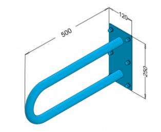
Arch fixed wall for disabled people, length 500 mm. generalpurpose, made of polished stainless steel tube or matt 32 mm diameter. We use this type of handrail in the washbasin, shower, and toilet area.
