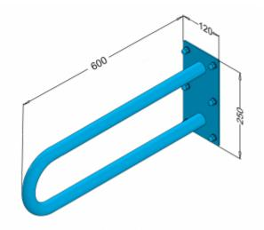
Arch fixed wall for disabled people, length 600 mm. generalpurpose, made of polished stainless steel tube or matt 32 mm diameter. We use this type of handrail in the washbasin, shower, and toilet area.
