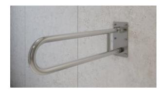
Arch hand-tilt, wall, for disabled people, 700 mm long, generalpurpose, made of polished stainless steel tube or matt 32 mm diameter. We use this type of handrail in the washbasin, shower, and toilet area.
