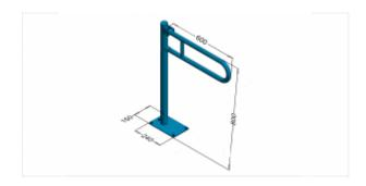
Arched, tilting handrail, adapted for floor mounting, for general use by the disabled. The handrail is made of AISI 304 stainless steel. The tube used for production has a diameter of 32 mm and a wall thickness of 1.5 mm. The total length of the curved railing is 600 mm, while the height of the supporting tube used is 800 mm. The steel handrail with a diameter of 32 mm, type 760, is available in two finishes:
