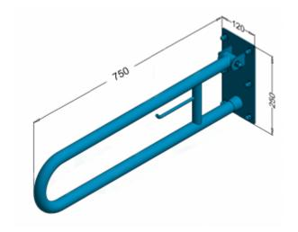
Tilting arch handrail with a place for toilet paper for disabled people, length 750 mm, general-purpose, made of polished stainless steel tube or matte 32 mm diameter. We use this type of handrail in the wc area.
