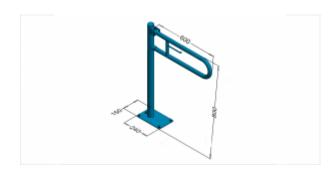
The handrail 760P is made of AISI 304 stainless steel. The tube used for production has a diameter of 32 mm and a wall thickness of 1.5 mm. The total length of the curved railing is 600 mm, while the height of the supporting tube used is 800 mm. The steel handrail with a diameter of 32 mm, type 760, is available in two finishes:
